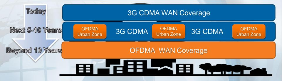
3G CDMA WAN networks will coexist with OFDM-based solutions until next generation 4G broadband networks are fully capable of delivering: Ubiquitous coverage Carrier-grade VoIP Low-cost devices Global roaming
