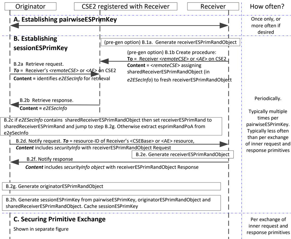
**Figure 11.4.2-1: The transport details for establishing pairwiseESPrimKey and establishing sessionESPrimKey in the End-to-End Security of Primitives (ESPrim) Procedure. This message flow shows the sequence of events for Blocking Mode**
