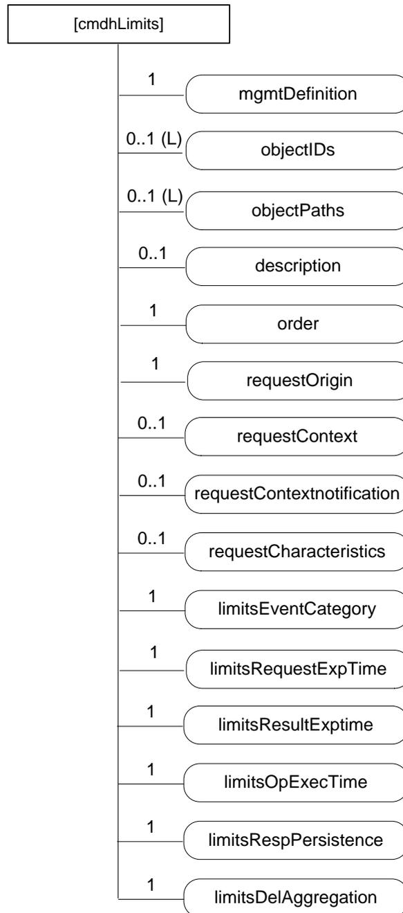
Figure D.12.5-1: Structure of [cmdhLimits] resource
