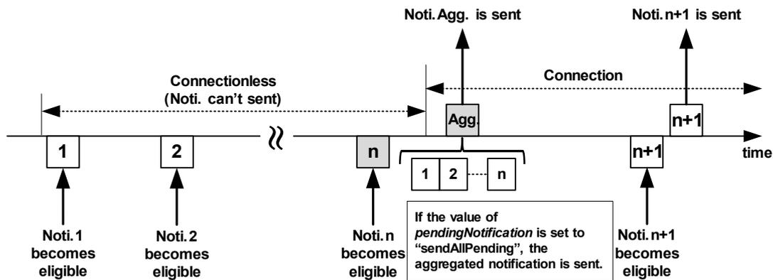
**Figure 10.2.12.1-2: Notification Mechanism when pendingNotification (sendAllPending) is used**
