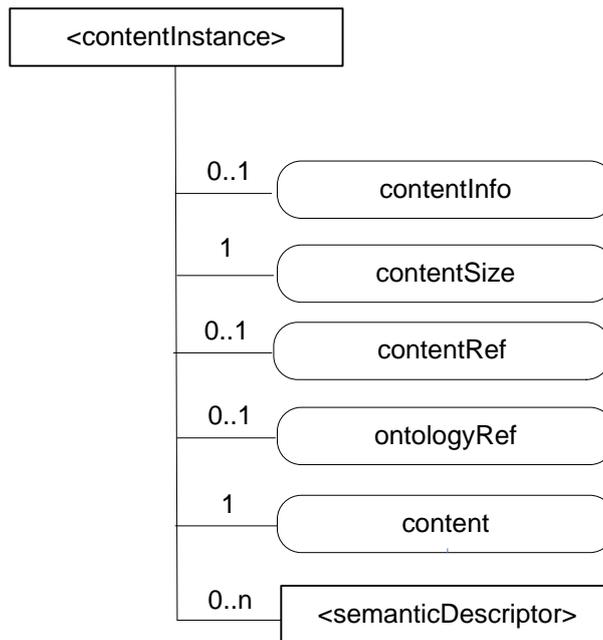
**Figure 9.6.7-1: Structure of *<contentInstance>* resource**
