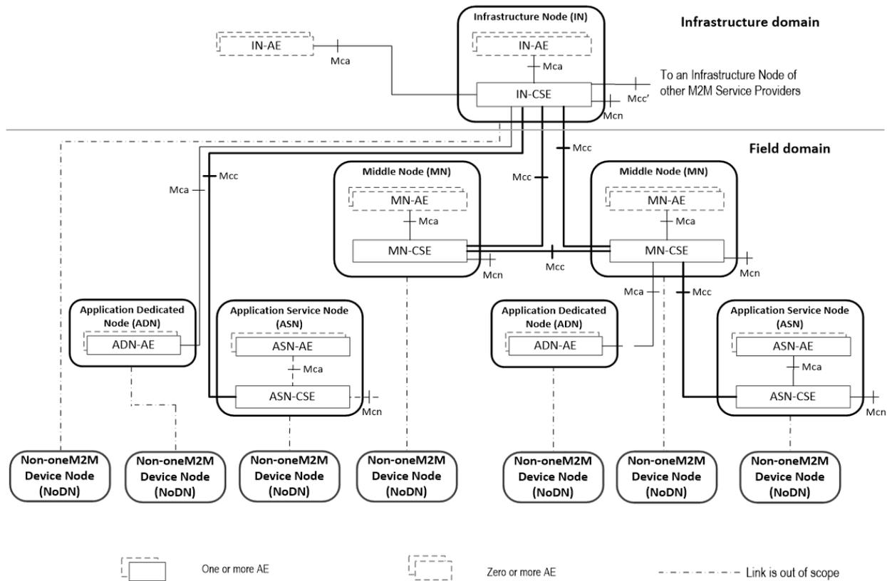
**Figure 6.1-1: Configurations supported by oneM2M Architecture**
