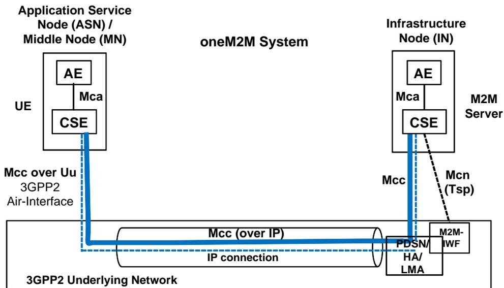
Figure C.4-1: User Plane and Control Plane Communication Paths
