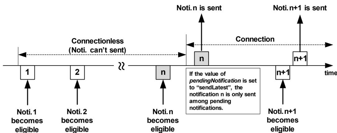
Figure 10.2.12.1-1: Notification Mechanism when *pendingNotification* (sendLatest) is used
