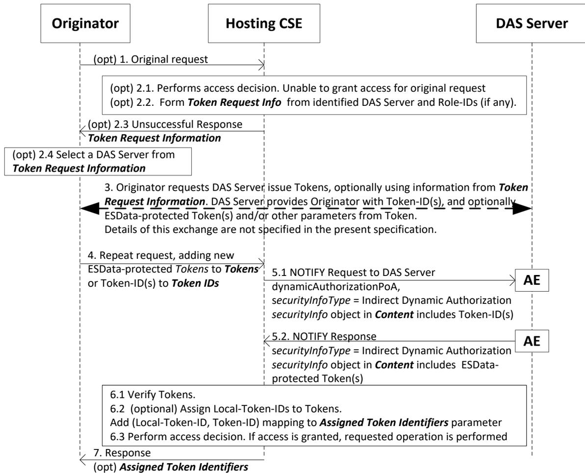
**Figure 11.5.3-1: Message flow for Indirect Dynamic Authorization**
