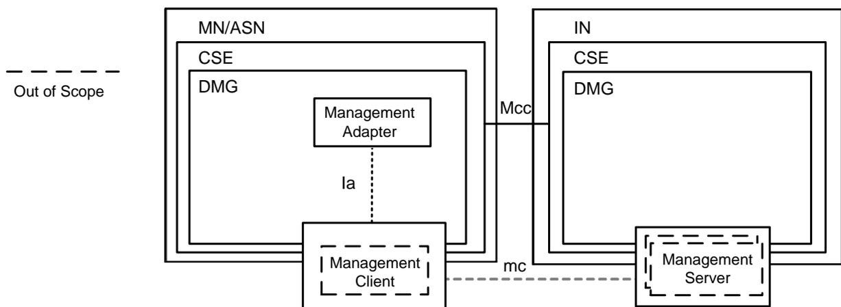
**Figure 6.2.4.1.3.1-1: Management Client Interaction using "la" interface**
