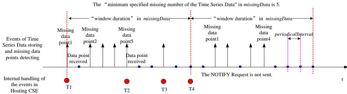
**Figure 10.2.39-1: Time Series Data Detecting and Reporting Mechanism**
