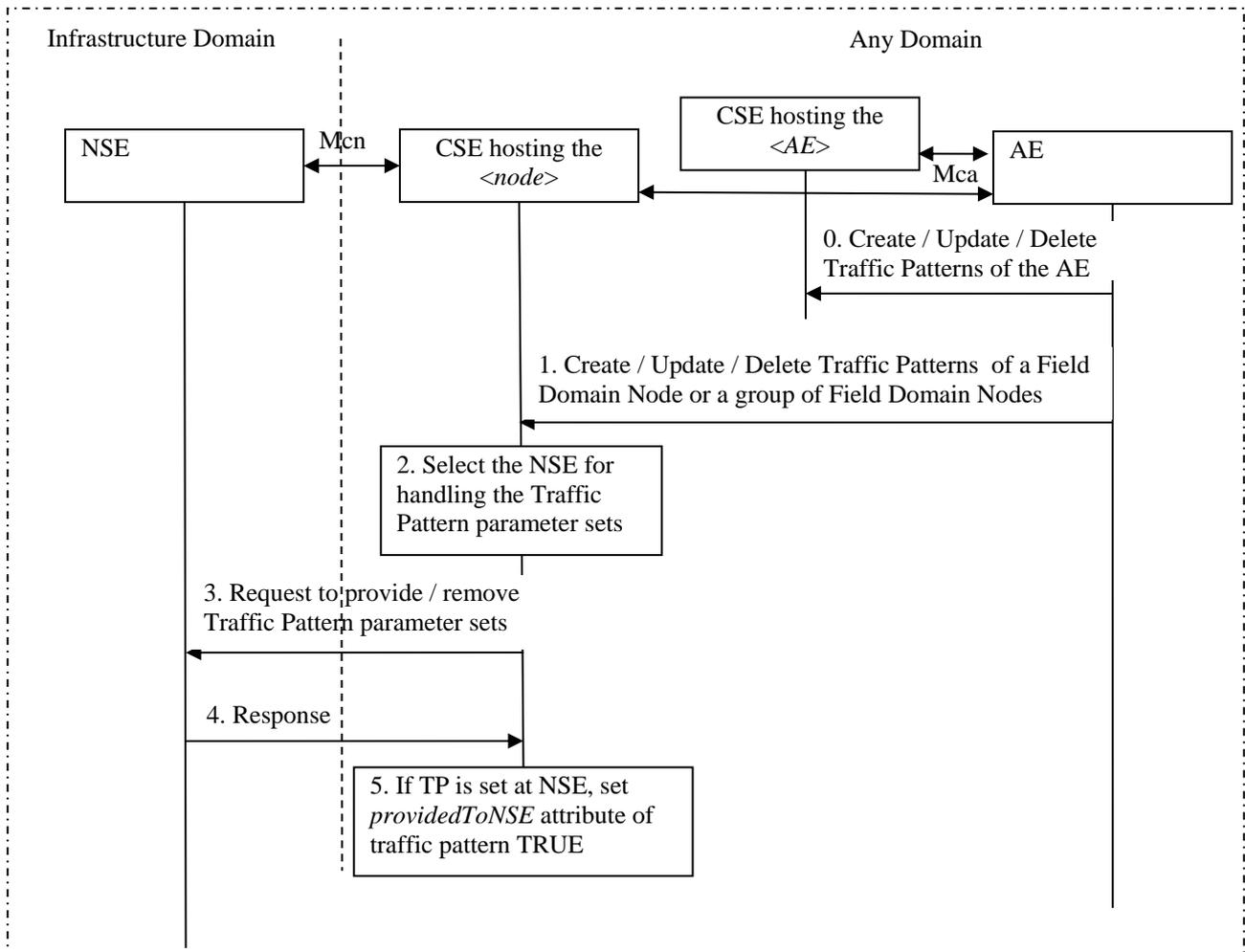
**Figure 8.3.5.3-1: General procedure for configuration of Traffic Patterns**
