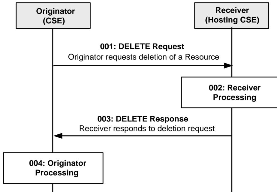
**Figure 10.1.4.2.1-1: Procedure for DELETING a <remoteCSE> Resource**
