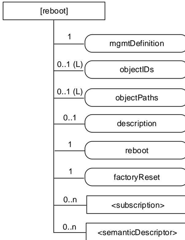
**Figure D.10-1: Structure of *[reboot]* resource**
