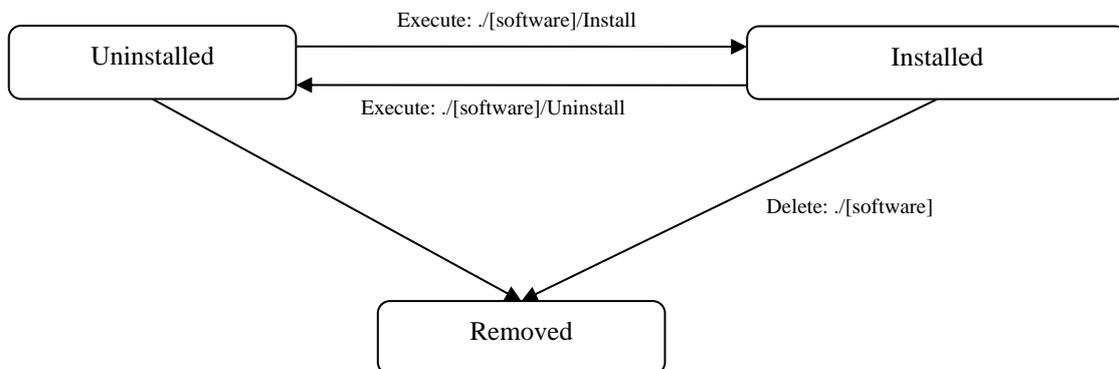
**Figure D.3-2: State machine for *[software]* management**
