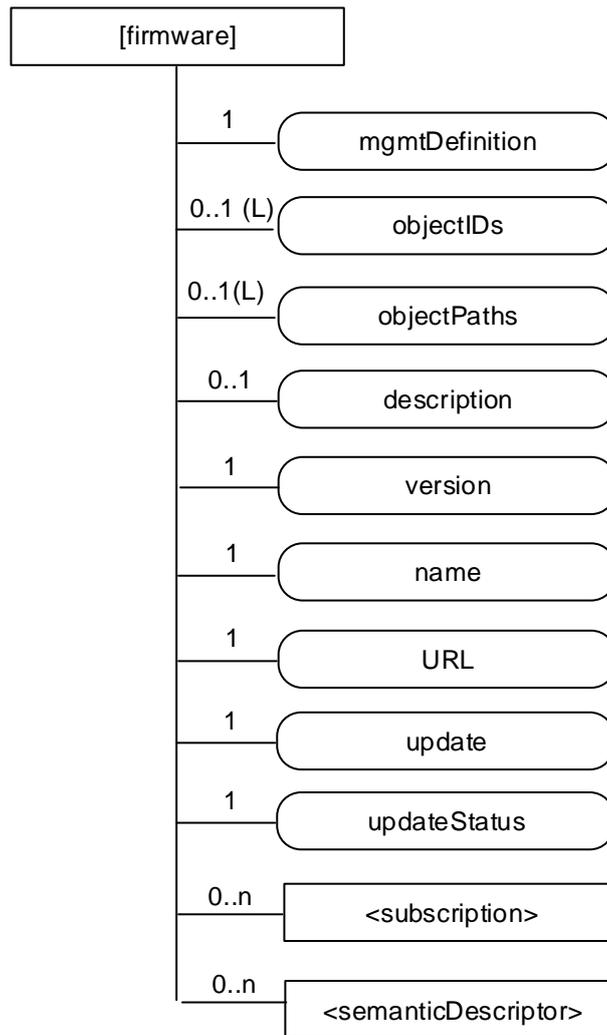
**Figure D.2-1: Structure of [firmware] resource**
