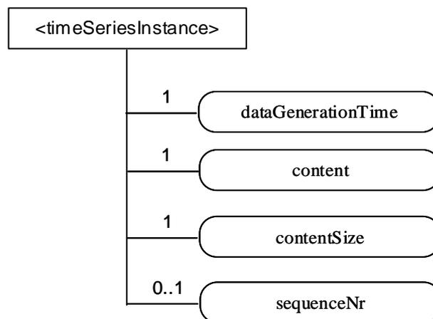
Figure 9.6.37-1: Structure of <timeSeriesInstance> resource
