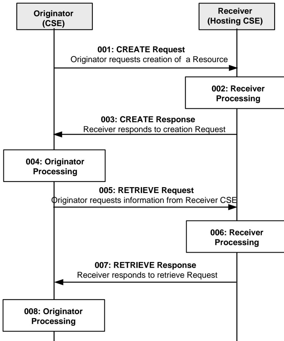
Figure 10.1.1.2.1-1: Procedure for CREATEing a <remoteCSE> Resource
