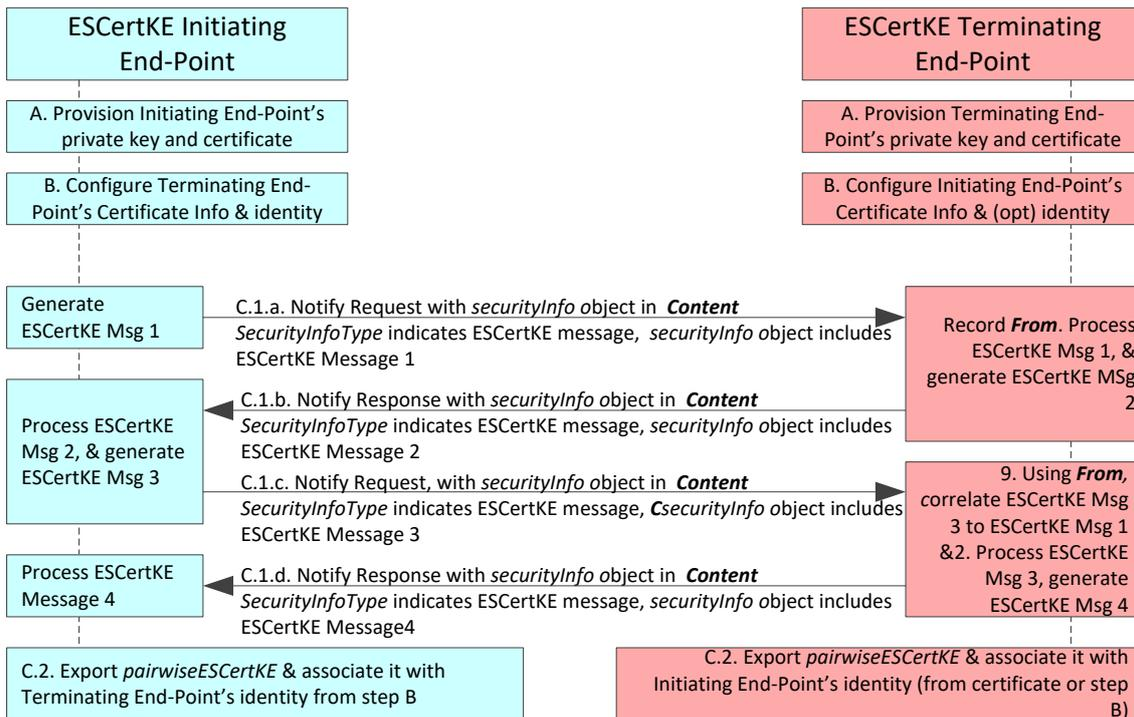
**Figure 11.4.3-1: The transport details for the ESCertKE Procedure**
